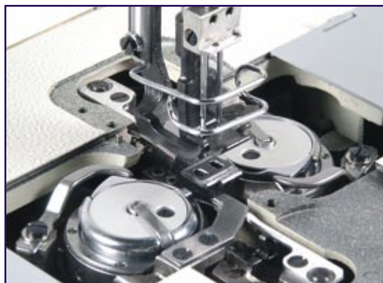
Thread trimming device and large hooks.
