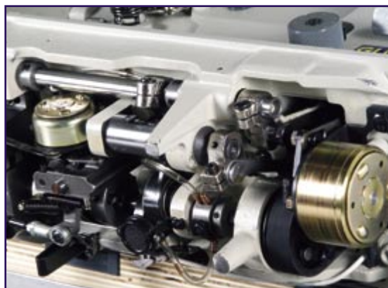
Solenoids for automatic thread trimming and back tack
