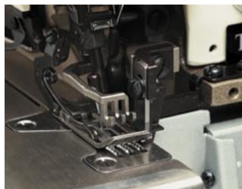
OV636-555 - 5 thread heavy duty top feed
