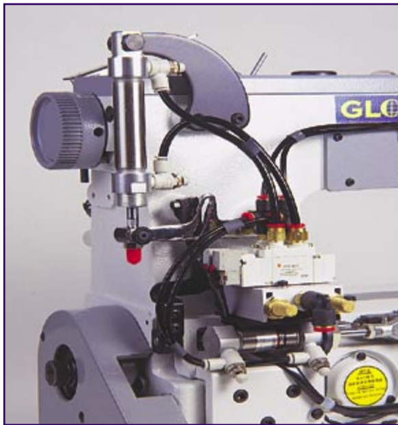
Pneumatic thread trimming and presser foot device
